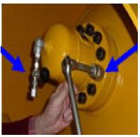
The patented C+S safety barrel for hydrogen chloride gas has two safety pressure lids. In the event of a leak in the valve area, these can be sealed gas-tight up to 150 bar within a few minutes. The safety pressure lid enables quick action in the event of danger. Standard transport lids are used for transport, which are secured with 2 screws.
